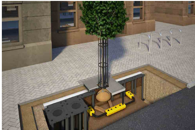
Figure 75: Linked Sustainable Drainage System. (SuDS) tree pit within the pavement. Tdag.
